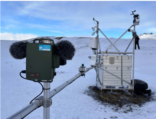
Figure 3: The Solander’s Eye field station with a mounted AudioMoth.
